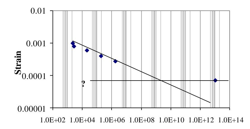
**Load Cycles to 50% Stiffness (Failure)**
